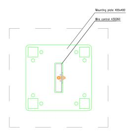
Recommended torque on bolt connection 10Nm.
